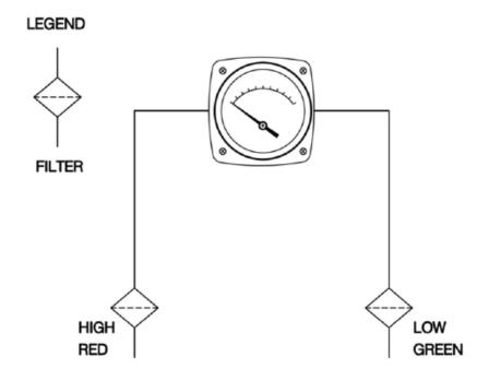
NOTE: This test kit is plumbed for water service. Contact the factory before using on other liquids or gases.
