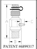
Combination manual air vent and pressure/temperature test port with brass body, dual durometer EPDM core, blowout-proof stem, side discharge vent with 1/8" (4mm) hose barb, threaded brass cap with O-ring seal and neoprene retainer strap. Accepts standard 1/8" (4mm) gauge adapter or thermometer stem.
